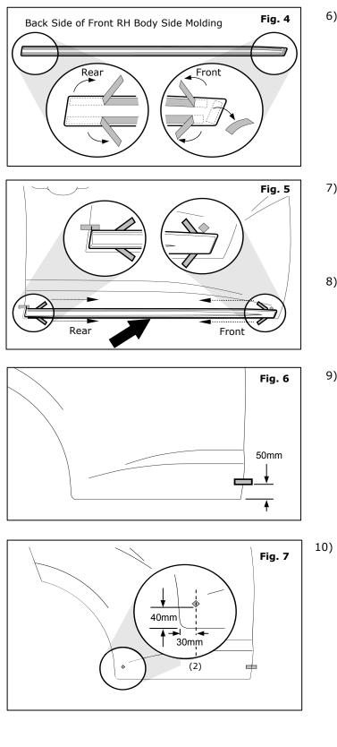
6) Remove tape liner from small tape. Peel back two long tape liners 30mm from each end of molding and fold them as shown **(Fig. 4)**
